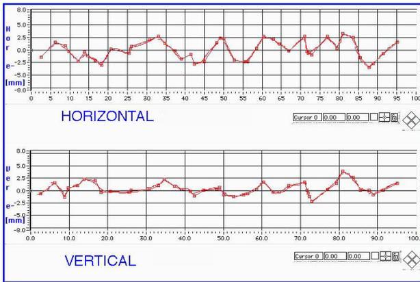
Figure 4: Corrected closed orbit in  $e^-$  ring
