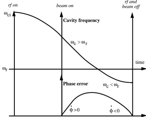
Fig. 6 : cavity frequency and phase error during filling time and beam pulse
