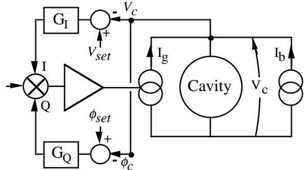
Fig. 4 : Schematic of the SOLEIL feedback system.
