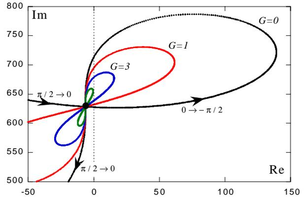
Fig. 5 : Root locus with  $\psi$  as variable for different loop gains  $G$  ( $Q=5 \cdot 10^6$ ,  $E_a=6\text{MV/m}$ ,  $f_m=100\text{Hz}$ ,  $Q_m=50$ ,  $k_m=2 \text{ Hz}/(\text{MV/m})^2$ )
