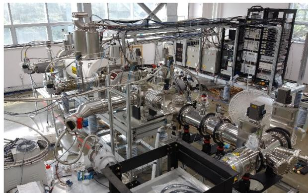
Figure 1: RAON EBIS charge breeder installed at Korea University Sejong.
