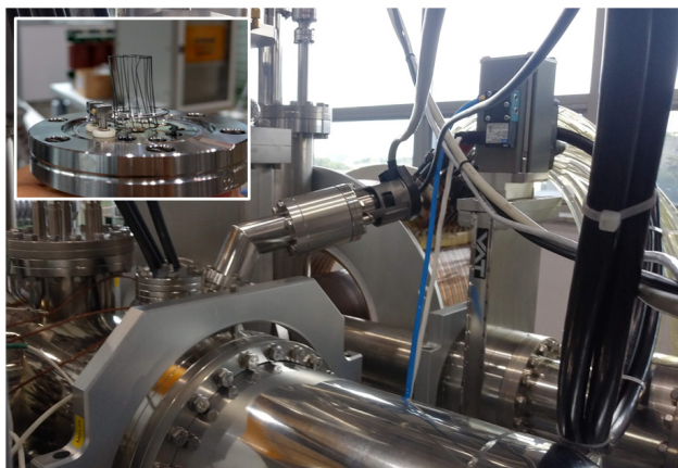
Figure 2: Ion gauge aligned to the magnetic line using the bent nipple. The inset shows the damaged inner structure of the ion gauge under a strong magnetic field.
