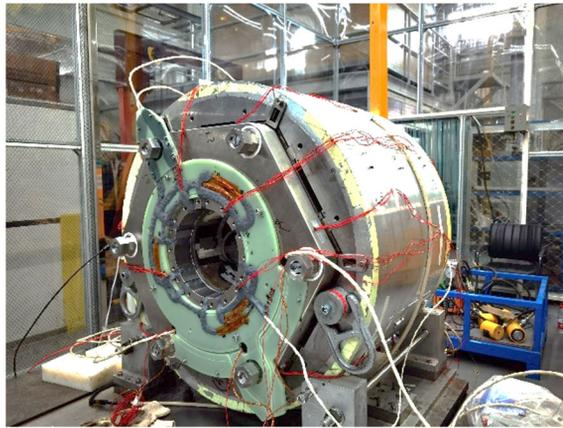
Figure 5: Picture of completed FECCR 1/2 size prototype cold mass ready for test.
