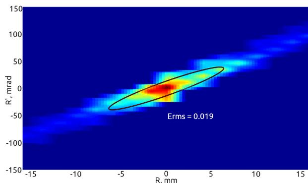
Figure 4: Emittance diagram example, obtained at a hydrogen pressure of 1 mTorr, 2 kW of microwave power and 30 kV of extraction voltage.
