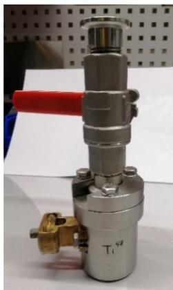
Figure 7: Container with  $(\text{CH}_3)_5\text{C}_5\text{Ti}(\text{CH}_3)_3$ .
