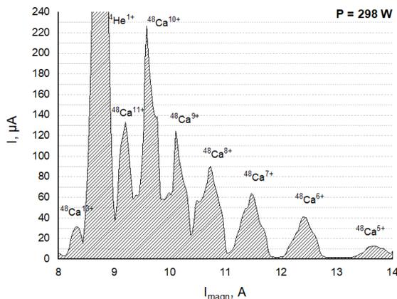
Figure 6: The  $^{48}\text{Ca}$  ion spectrum, optimized for  $\text{Ca}^{10+}$ .
