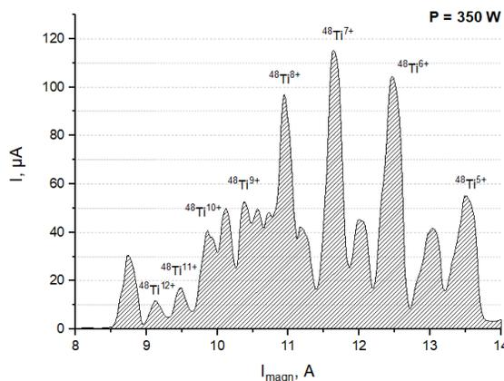
Figure 8: The  $^{48}\text{Ti}$  ion spectrum, optimized for  $\text{Ti}^{7+}$ .
