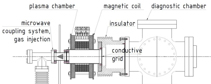
Figure 1: The principal scheme of the constructed experimental bench.
