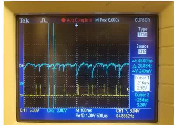
Figure 3: (Top) Two test measurements were performed: one where a TTL was output immediately after the instability event, within  $0.667 \mu\text{s}$ , and one where the TTL was delayed by 8 ms. (Bottom) Example picture of showing the TTL output along side the measured  $\text{O}^{6+}$  beam current, on an oscilloscope.
