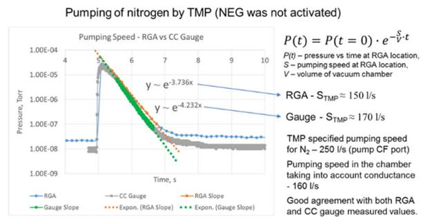
Figure 10: Pumping speed of nitrogen by TMP measured by RGA (blue dots and line, red line – approximation by exponential function) and CC gauge (grey line, green line – approximation by exponential function).
