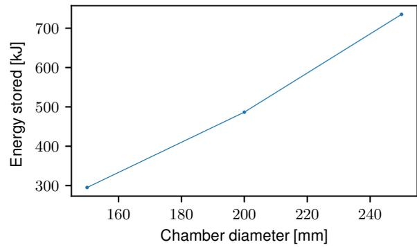
Figure 6: Magnetic energy stored in the system for different plasma chamber diameter.
