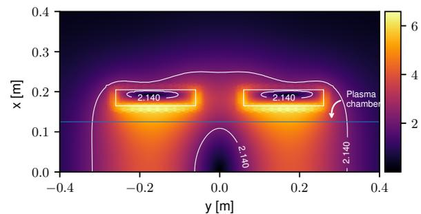
Figure 3: Field map for 250 mm diameter plasma chamber. Plasma chamber (blue). Surface of 2.14 T
