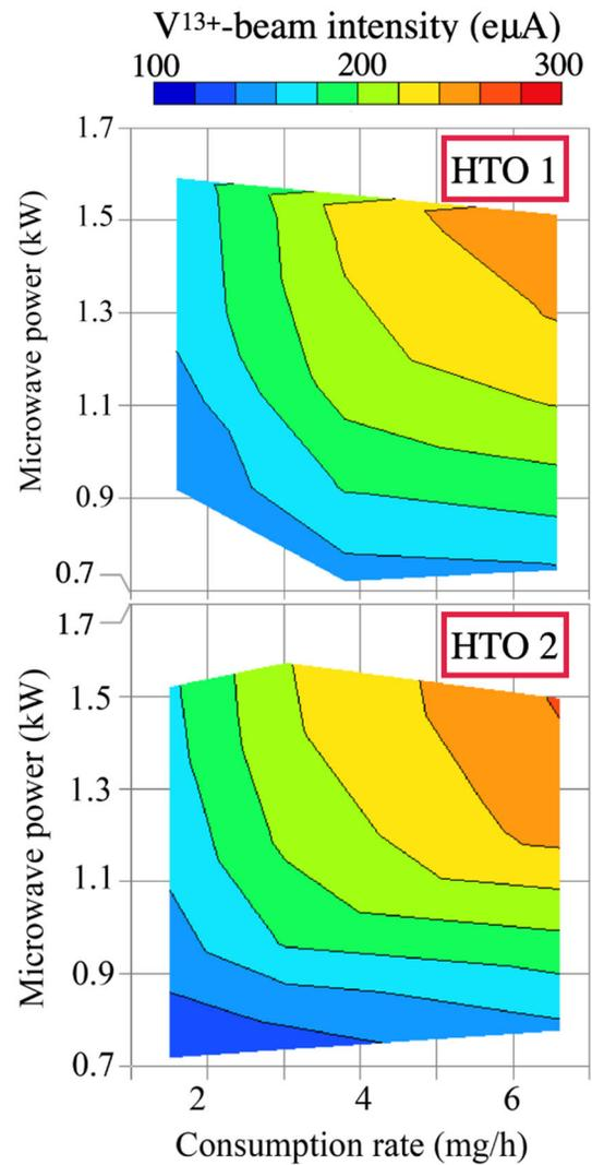
Figure 2: Obtained contour plots of the  $^{51}\text{V}^{13+}$ -beam intensity as a function of the total power of the 18- and 28-GHz microwaves and consumption rate of the V sample using HTO 1(top) and HTO 2 (bottom).
