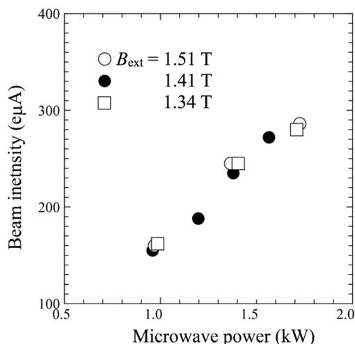
Figure 5: Beam intensity of  $V^{13+}$  as a function of microwave power for mirror fields for extraction regions  $B_{ext}$  of 1.51 T (open circles), 1.41 T (closed circles), and 1.34 T (open squares).
