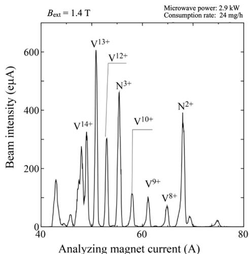
Figure 4: A mass-to-charge-ratio spectrum was obtained with a total microwave power of 2.9 kW and a consumption rate of 24  $\mu g/h$
