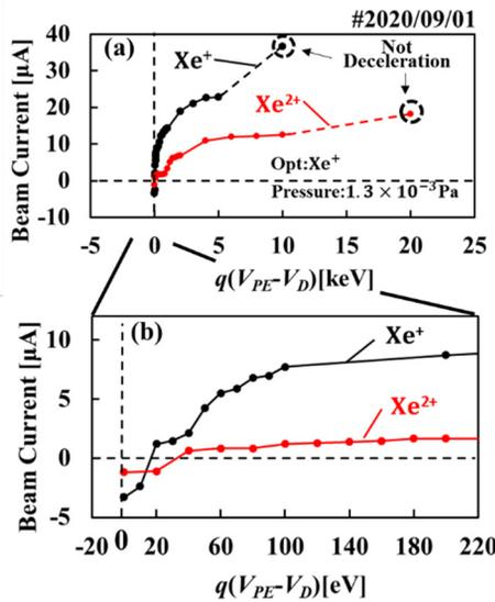
Figure 5: Xe deceleration experiment.
