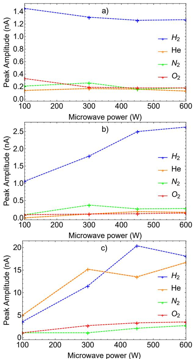
Figure 4: Evolution of a) <sup>40</sup>Ar<sup>7+</sup>, b) <sup>96</sup>Mo<sup>15+</sup> and c) <sup>12</sup>C<sup>5+</sup> peak amplitude as a function of microwave power and CB support gas plasma species.
