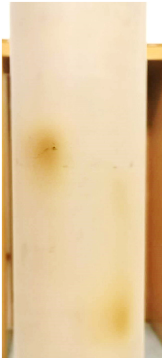
Yellowish PEEK insulator after high power operation (1.5 mm Ta shielding)
