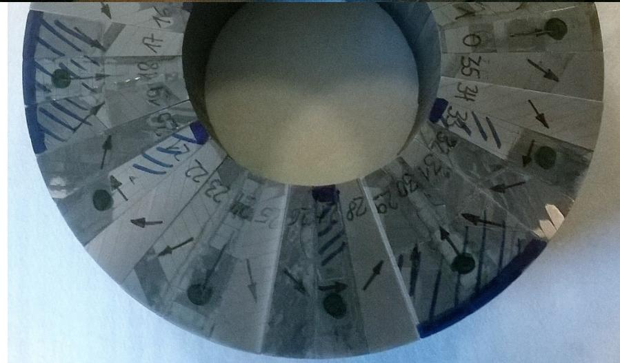
**Grain boundary diffusion process to enhance coercivity on both materials to avoid demagnetization issues**
