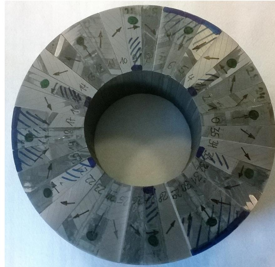
**Grain boundary diffusion process to enhance coercitivity on both materials to avoid demagnetization issues**
