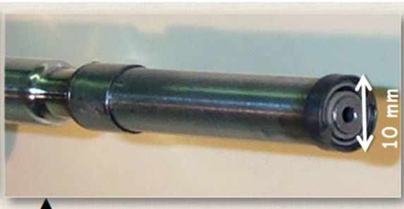
The Large Capacity Oven to evaporate SiO , WO_3 and Te
