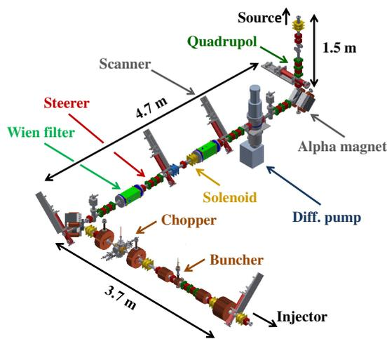
Figure 1: Layout of the low energy beam transport system for MESA.
