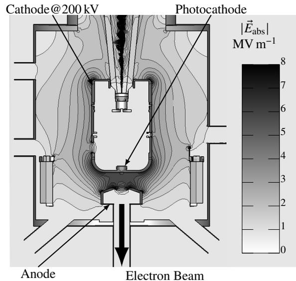
Figure 2: Electrostatic simulation using CST. The absolute field gradient in STEAM @  $U = 200 \text{ kV}$  stays below  $10 \text{ MV m}^{-1}$ , while an extracting field gradient of  $|\vec{E}_{\text{acc}}| \approx 5 \text{ MV m}^{-1}$  is achieved. The HV cable is also simulated.
