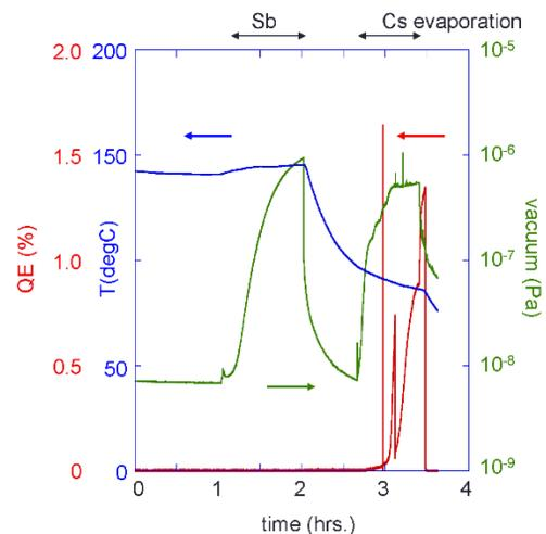
Figure 1: The Cs<sub>3</sub>Sb photocathode fabrication procedure. The blue curve shows temperature of puck holder measured with a thermocouple. The green curve shows the vacuum pressure in the fabrication chamber. The antimony is evaporated at the monitor temperature of 140-degree C and caesium is evaporated at 90-degree C. The QE (red curve) is derived from photo current measured with a charge collector in front of a Cs<sub>3</sub>Sb photocathode and laser power at 532 nm.
