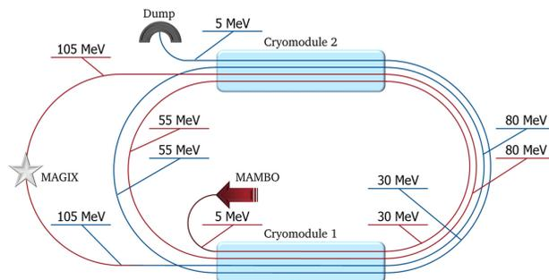
Figure 2: Sketch of the way a beam travels through MESA in the energy-recovery mode. Red: accelerating phase. Blue: decelerating phase. Note that the spatial separation is meant to clarify the different ways—in reality, the bunches are interleaved and those with the same energy share also the same beampipes in the arcs.
