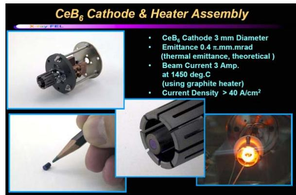
Fig. 3: CeB<sub>6</sub> single crystal thermionic cathode for low emittance electron source.
