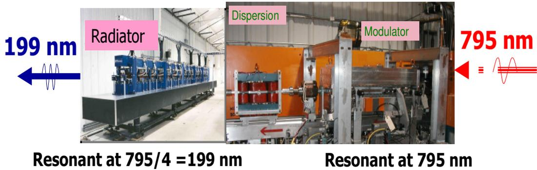
Figure 1: The SDL HGHG magnets and schematic of the 4<sup>th</sup> harmonic HGHG.
