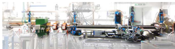
Figure 1: The SPARC photoinjector in the initial phase: from the right to the left, the RF gun with the solenoid, the emittance meter, quadrupoles and dipole magnets, the energy spectrometer and the beam dump.
