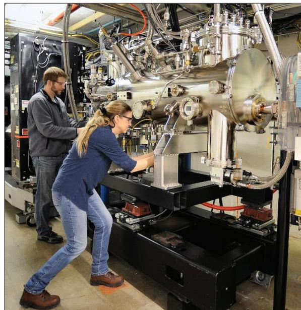
Figure 2: Helical SCU installed in Sector 7.
