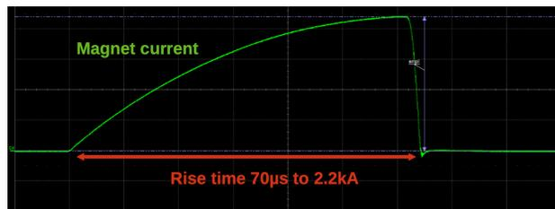
Figure 1: Pulse shape of the injection kickers.
