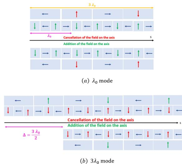
Figure 1: Configuration of magnet magnetization.
