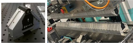
Figure 5: Module of magnets (left) and prototype installed on magnetic measurement bench (right).
