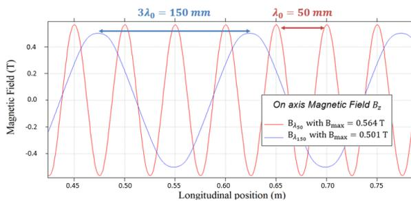
Figure 3: One axis magnetic field  $B_z$  at gap 15.5 mm:  $\lambda_0$  mode in red (50 mm period appears) and  $3\lambda_0$  mode in blue (150 mm period appears).
