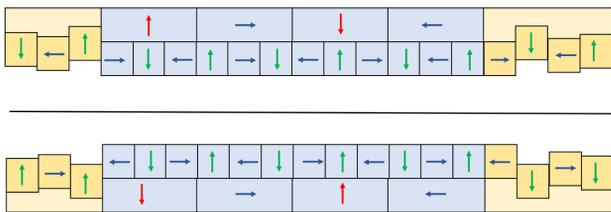
Figure 2: Configuration of magnets for the  $\lambda_0$  mode.
