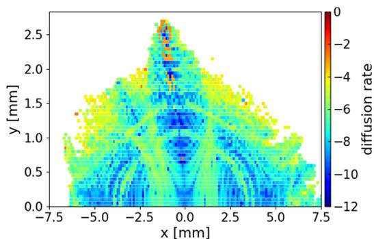
Figure 6: DA of the reference solution of the SOLEIL II TDR lattice, with colour bar indicating diffusion rate.
