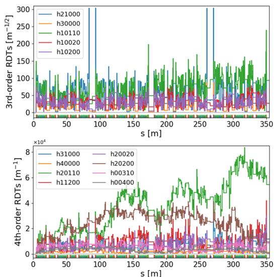
Figure 5: Fluctuation of 3<sup>rd</sup>- and 4<sup>th</sup>-order RDTs of the reference solution of the SOLEIL II TDR lattice.
