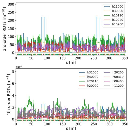
Figure 7: Fluctuation of 3<sup>rd</sup>- and 4<sup>th</sup>-order RDTs of one optimized solution.
