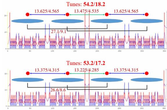
Figure 2: Simplified model for calculating low-frequency RDT fluctuations of the SOLEIL II CDR lattice with betatron tunes of 54.2/18.2 and 53.2/17.2.
