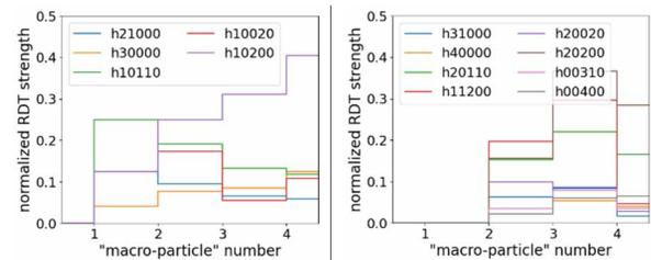
Figure 4: Low-frequency fluctuations of 3<sup>rd</sup>- and 4<sup>th</sup>-order RDTs for the betatron tunes of 53.2/17.2.
