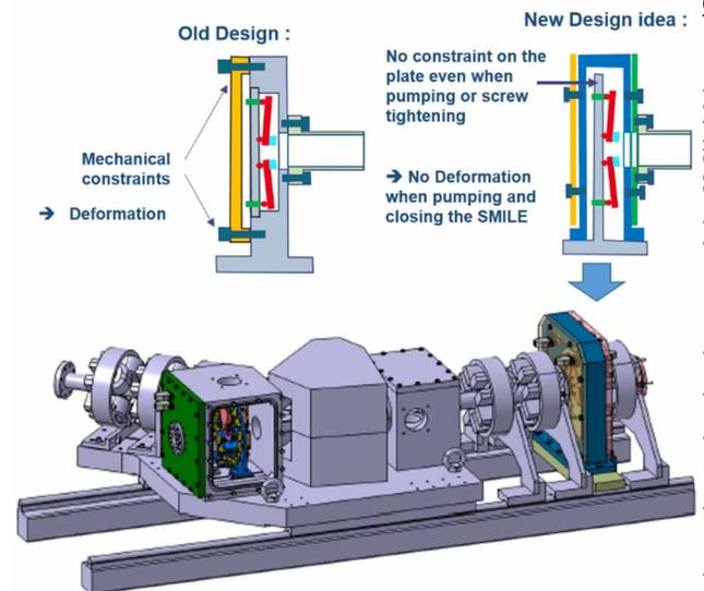
Figure 6: New mechanical design of the SMILE with better mechanical constraints management.
