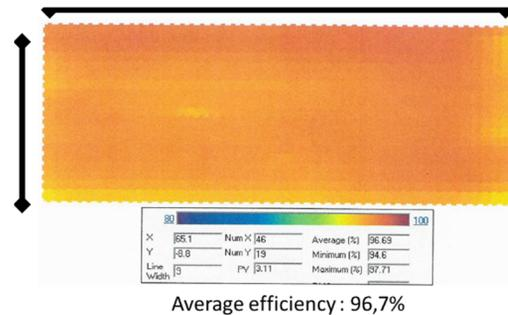
Figure 9: Scanning of the diffraction efficiency over the surface of the grating. Excellent efficiency was achieved. Courtesy: Plymouth Grating Laboratory
