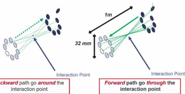
Figure 4: Trajectories of laser beams in the backward and in the forward direction.
