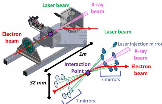
Figure 3: 3D view of the SMILE and schematic (not to scale) with highly exaggerated angle.
