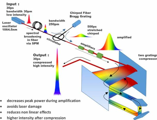
Figure 8: Principle of the new CPA system under development.
