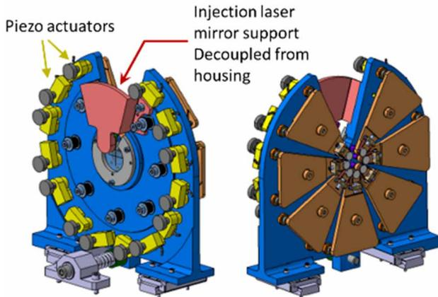
Figure 7: New design for the injection laser mirror and addition of piezo actuators
