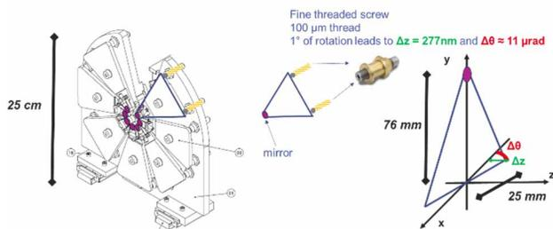
Figure 5: 3D view of the SMILE and schematic.
