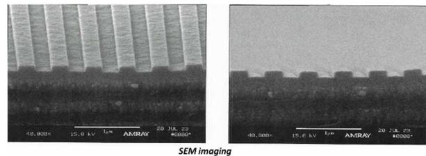
Figure 10: SEM imaging of the grating. Courtesy: Plymouth Grating Laboratory
