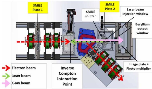
Figure 2: Top view of the Compton interaction Region.
