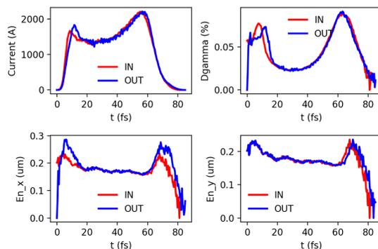
Figure 8: Comparison of beam parameters at entrance and exit of the bypass line.
