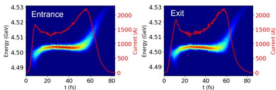
Figure 9: Phase space at entrance (left) and exit (right) of the bypass line.
