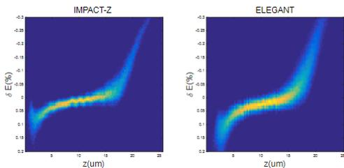
Figure 5: Phase space at exit of Linac with IMPACT-Z (left) and ELEGANT (right).
