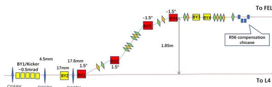
Figure 7: Layout of the bypass line.
