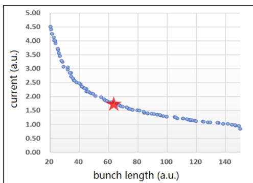
Figure 2: Pareto front of Linac longitudinal optimization.
