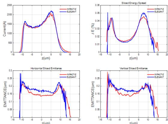
Figure 6: Final current distribution, sliced energy spread and normalized sliced emittance.
