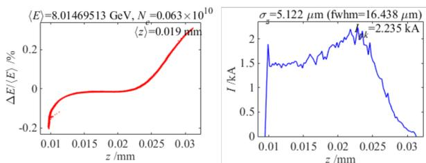
Figure 3: Longitudinal phase space (left) and beam current profile at the exit of Linac through MOEA.
