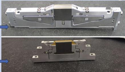
The first CPMU had only 4 columns. Upon cooling the CPMU it was found that four columns was too few to correct the device satisfactorily. The number of columns was increased to five for the subsequent CPMUs. Using an odd number of columns also meant that the centre columns could be fixed and the girders would contract equally around the centre columns upon cooling, rather than unequal contraction around the off-centre fixed columns of CPMU-1.
