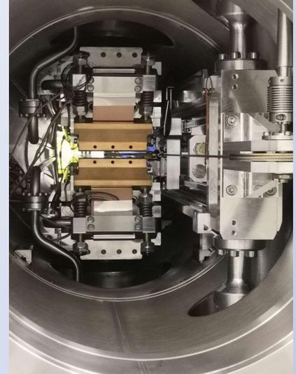
Above: the cold measurement system Hall probe beam installed in the vacuum chamber alongside CPMU-1. The pulley system with its coupling to the out-of-vacuum motor is visible on the right. On the left the LN<sub>2</sub> cooling pipes can be seen.
