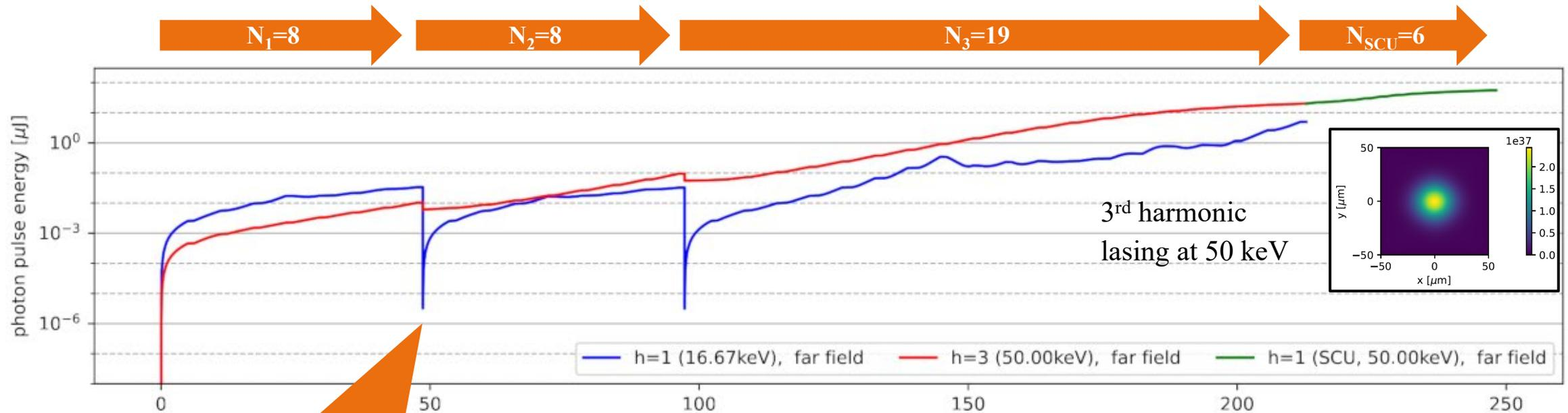
Disruption of the fundamental by a Si filter using the self seeding chicanes in SASE2
