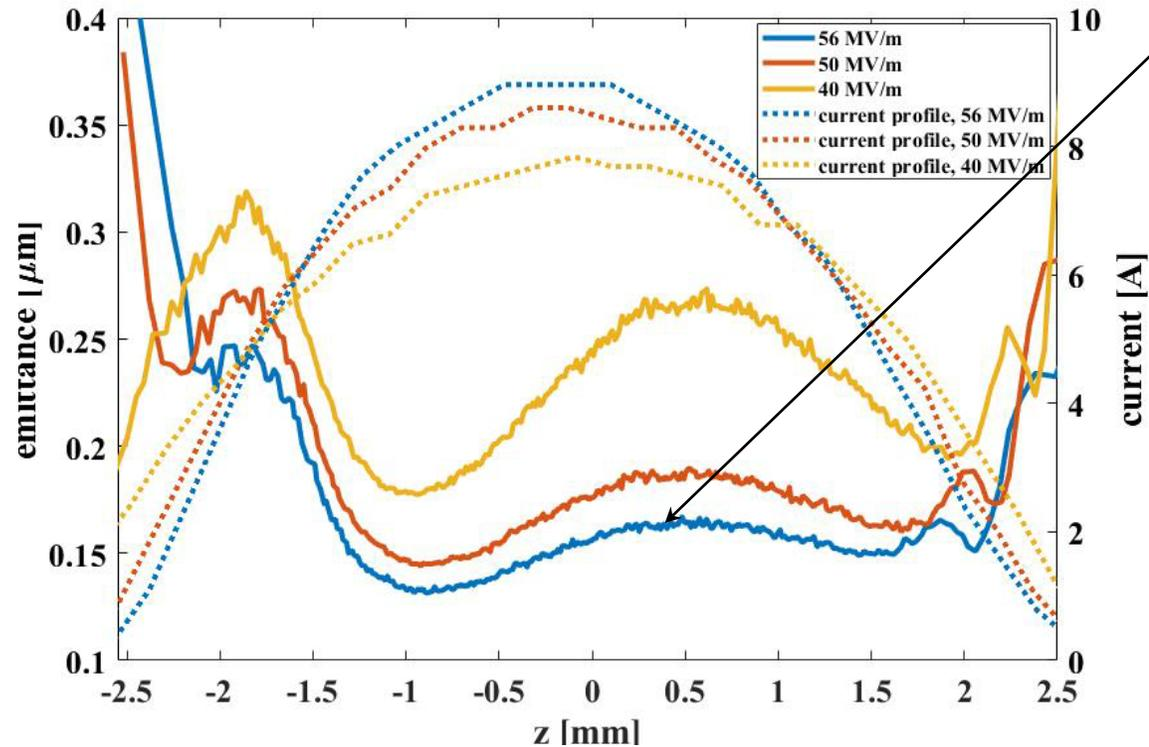
$\epsilon(\text{slice}) = \sim 0.16 \mu\text{m}$  at 56 MV/m
