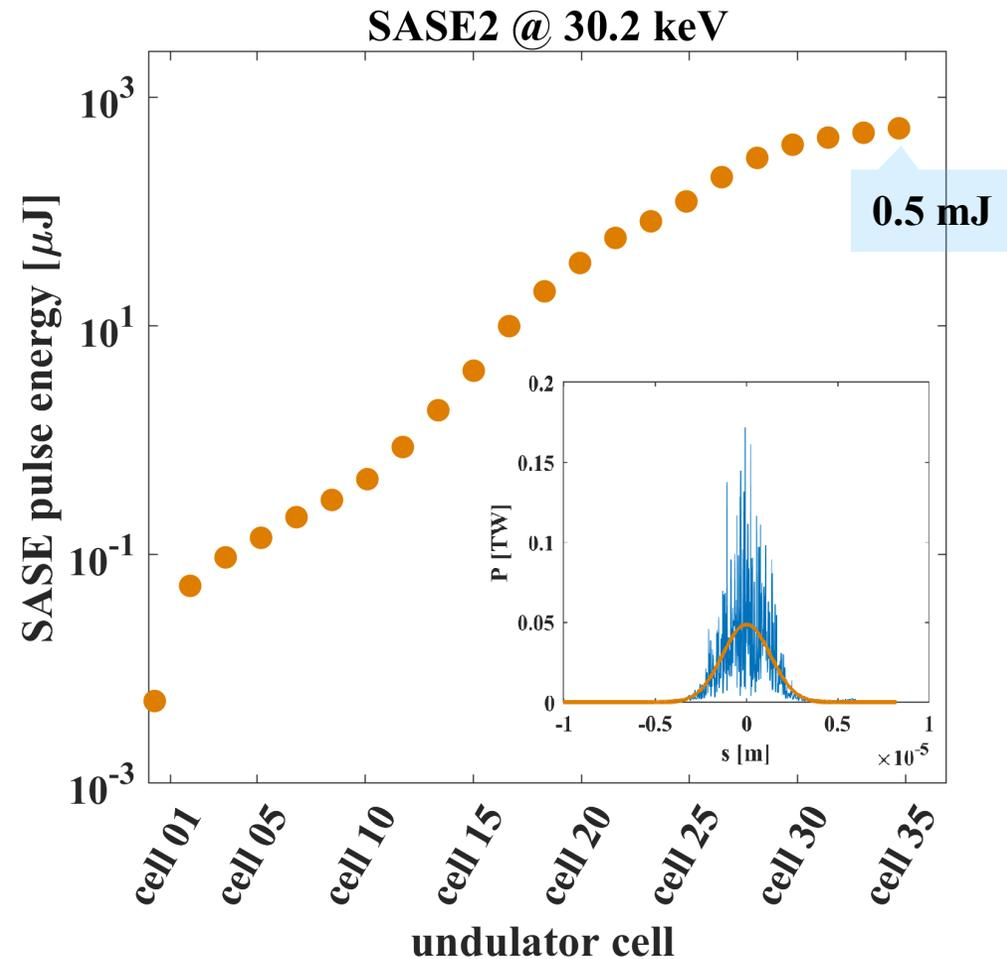
Simulated SASE intensities at 24.58 keV (left) and 30.24 keV (right) for beamlines SASE1 and SASE2. Linear & quadratic tapers optimized; No alignment error considered.
