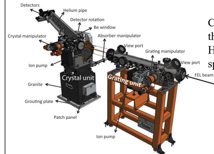
CAD model of the SASE1 HIREX spectrometer
