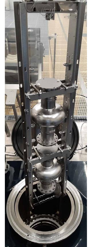
furnace installation of two R&D cavities
