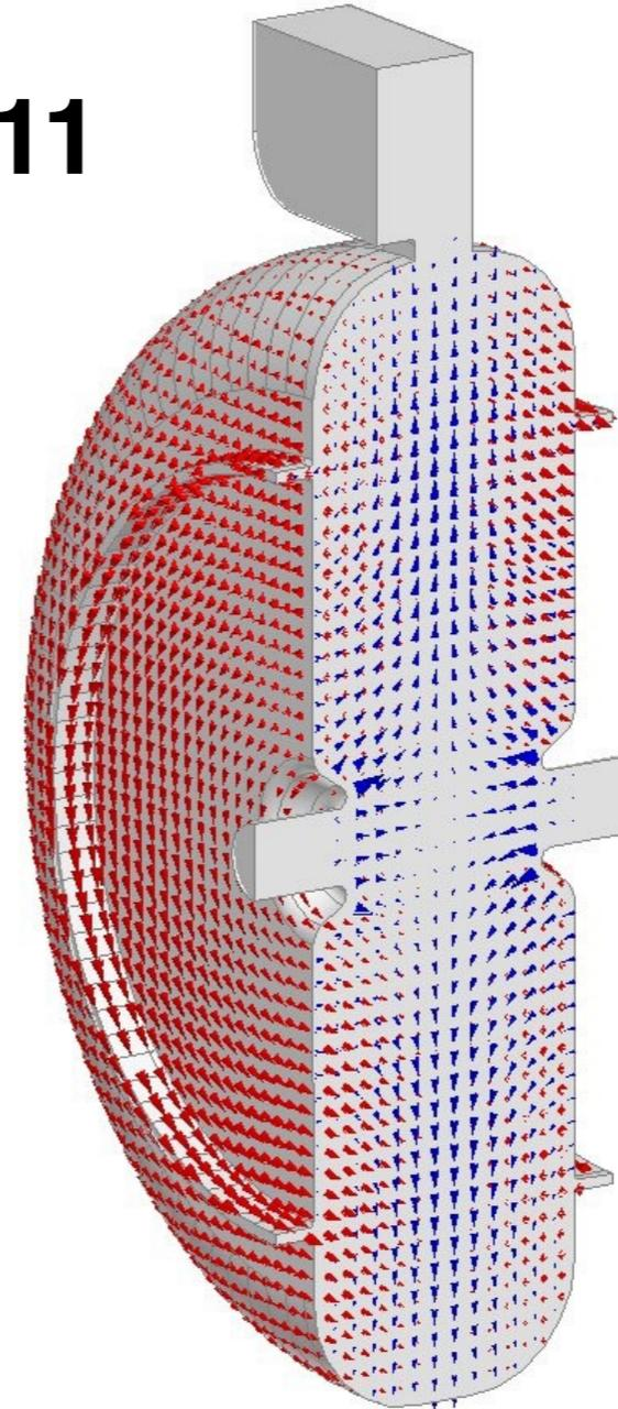
**Fields of monopole and dipole modes except TM020 mode get into the slots**
