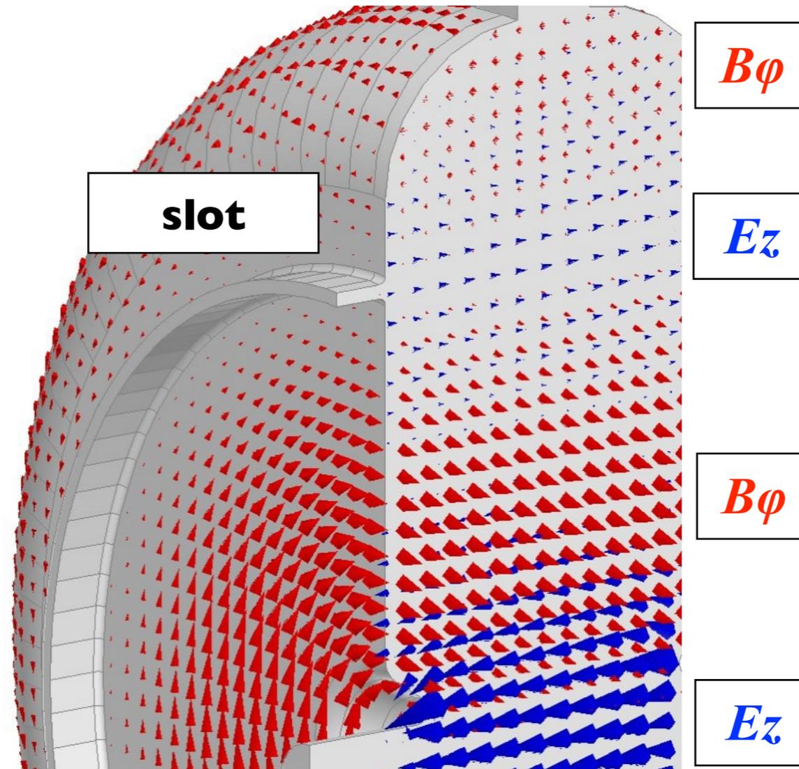
**Slots along the nodes of magnetic fields and parallel to electric fields
