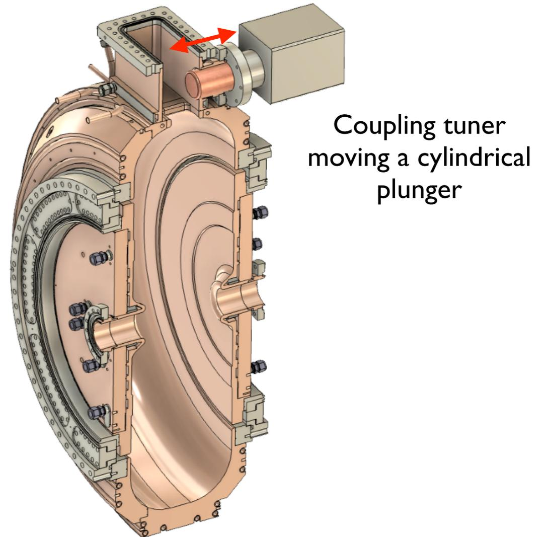
**Coupling  $\beta$  adjustable to the value best for beam loading during high-power operation in vacuum**
