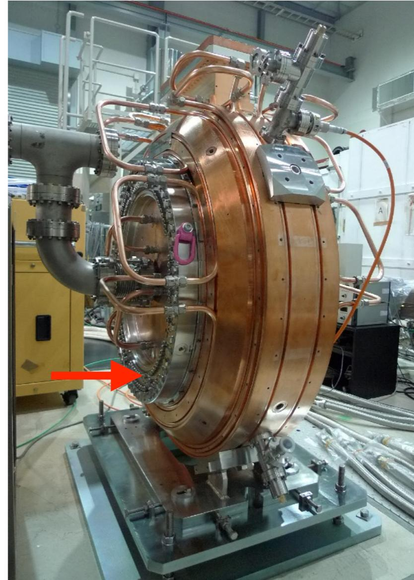
**16 HOM dampers directly embedded into the cavity body**
