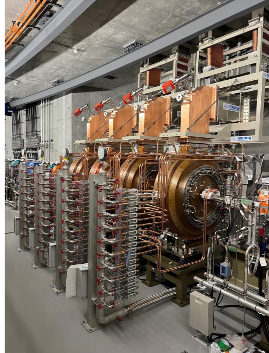
**Four cavities have begun to accelerate a beam**
