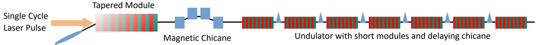
Alternatively a chirped laser pulse and a short modulator can be used.
