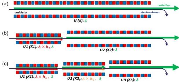
In planar undulators odd harmonics can also drive the FEL process albeit on a lower growth rate. However, the slippage is enhanced by the harmonic number, resulting in increased coherence length
