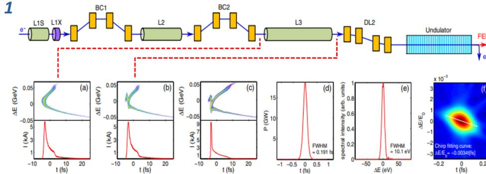
Electron beam is over-compressed with one leading current spike, driving the lasing. Performance is rather robust against RF jitter
