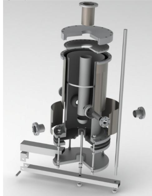
Figure 4: General view of 162 MHz QWR design model for  $\beta_g = 0.12$ , the RF frequency tuner is placed bottom of the cavity, the RF load loop and the measurement loop are not visible.
