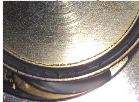
Figure 11: The picture above shows a damaged o-ring seal on a vacuum valve after being damaged by stray field emitted electrons.
