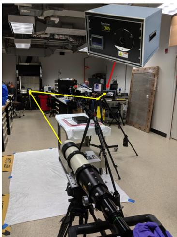
Figure 7: Using the blackbody source for calibration.
