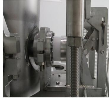
Figure 8: Adjustable  $Q_e$  coupler structure for HWR cavity vertical test.
