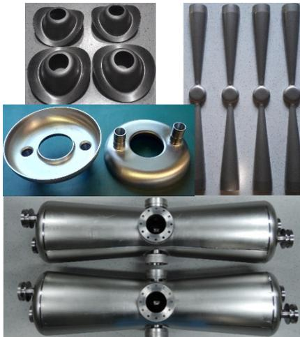
Figure 7: Fabrication of  $\beta_g=0.09$  HWR cavity.
