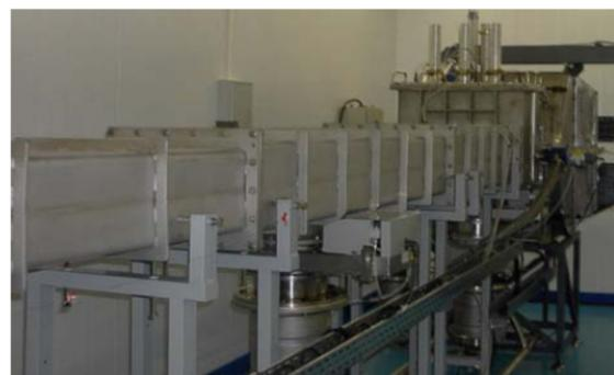
Figure 13: TM beam line of IC100 cyclotron [4].
