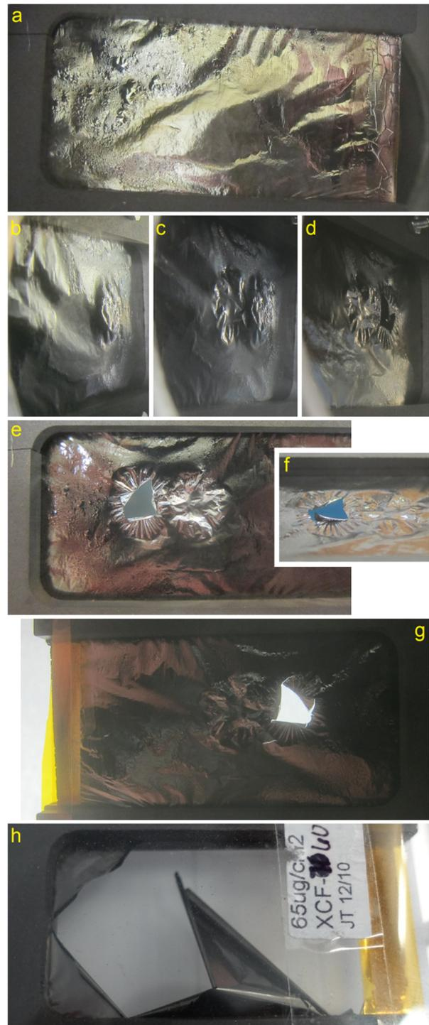
Figure 4: a) Foil before irradiation. b-d) After 1<sup>st</sup>/2<sup>nd</sup>/3<sup>rd</sup> fraction, in vacuum. e-g) Afterwards in air. h) Other foil, damaged at mounting. a,e,f,h) front, b-d, g) rear side.
