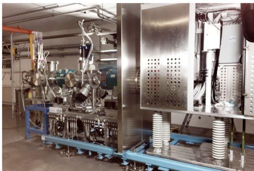
Figure 5: IS and LEBT installed in the ESS linac tunnel.
