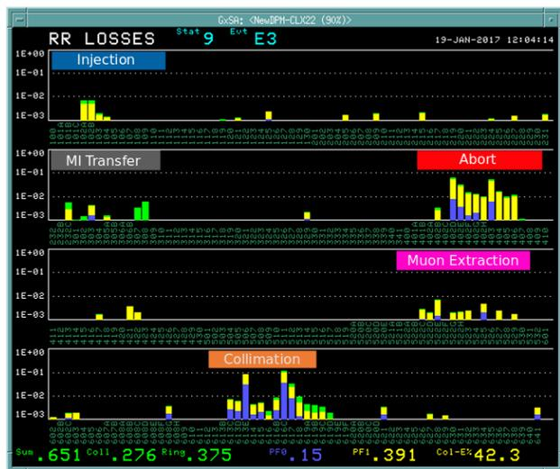
Figure 7: Typical loss pattern after the implementation of the the slip stack damper which allowed chromaticity to dropped at the end of the cycle. Intensity is around 45E12 ppp.
