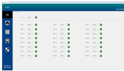
Figure 9: CSS OPI screen of the fast protection system.
