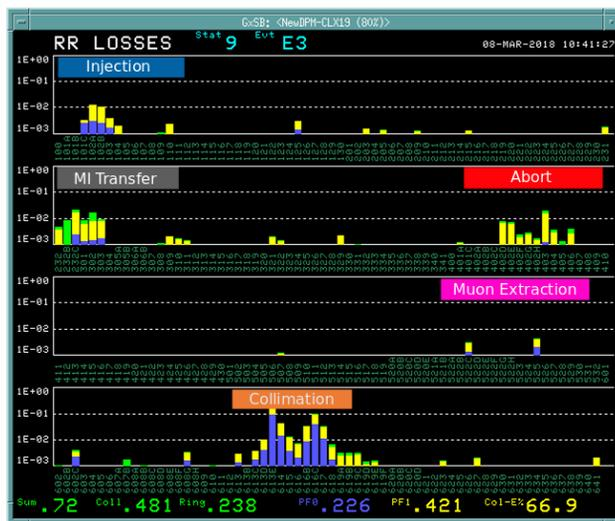
Figure 9: A typical loss pattern after the aperture improvements. Intensity is around 50E12 ppp.
