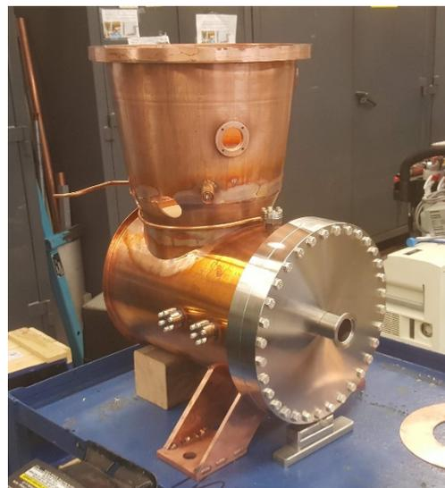
Figure 13 : The partially assembled cavity.
