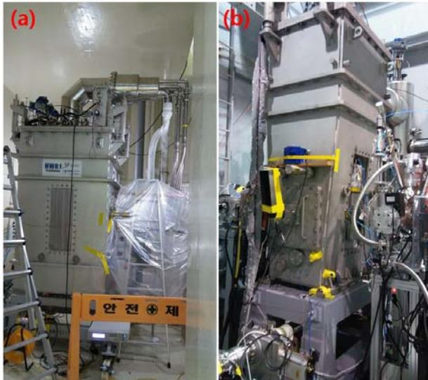
Figure 6: Cryomodules for (a) HWR and (b) QWR.
