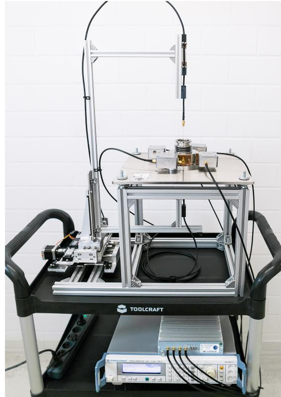
Figure 1: View of the BPM test bench with Libera Spark for data acquisition.
