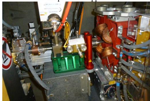
Figure 2: BLMs in undulator intersection.
