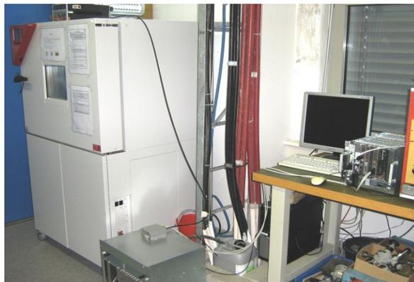
Figure 1: Climate cabinet with dose measurement setup.
