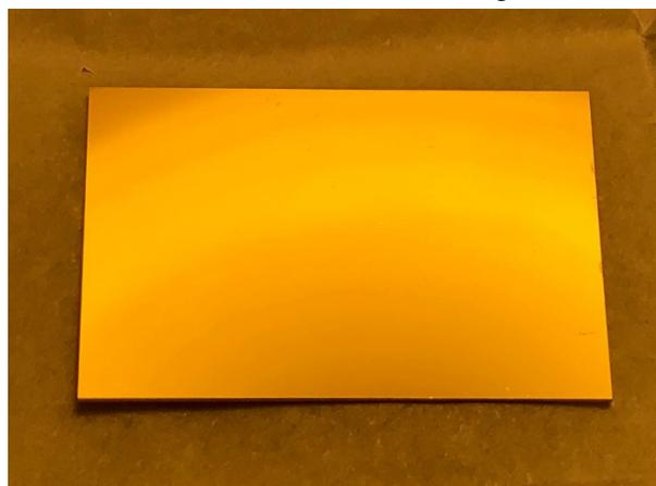
Figure 1: A 20 mm x 30 mm x 0.5 mm diamond mirror, consisting of six 10 mm x 10 mm monocrystals fused together, with 3 μm Au reflective coating. The light intensity pattern seen on the mirror surface comes from the reflector of the lamp used to illuminate it.
