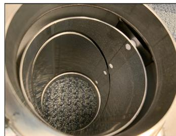
Figure 3: Picture of split-plate BPM implemented.
