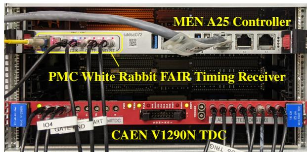
Figure 2: VMEbus mainframe configuration.
