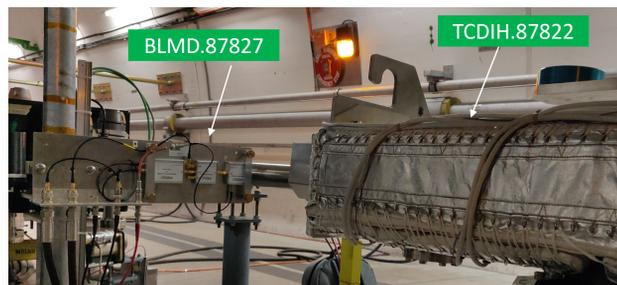
Figure 2: Photo of a dBLM detector installed at the end of the T18 LHC injection line.
