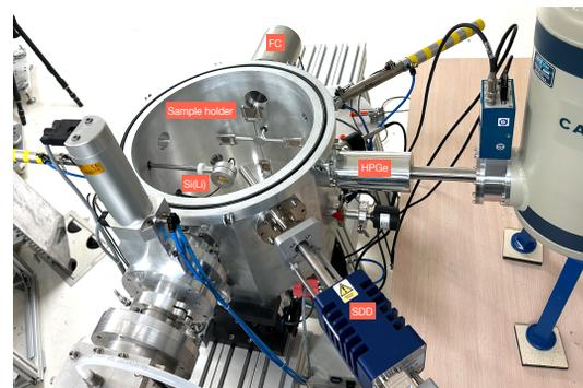
Figure 1: Irradiation system and detector placement.
