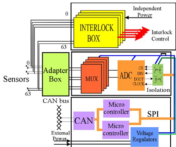
Fig. 3 Block diagram of the LMB
