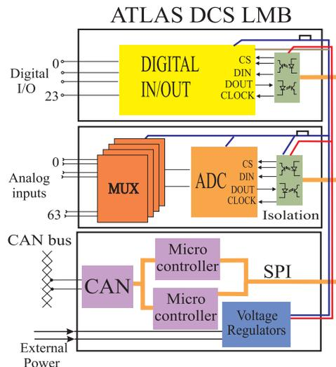
Figure 1 Block diagram of the LMB
