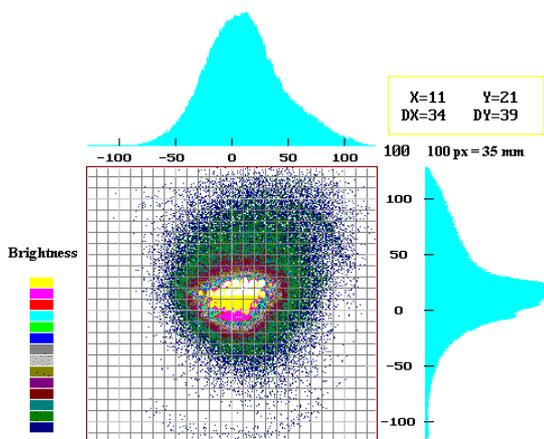
Figure 2: Beam image with X- and Y- profiles.
