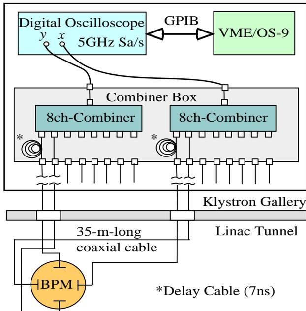
Figure 2: Schematic drawing of a front-end system.
