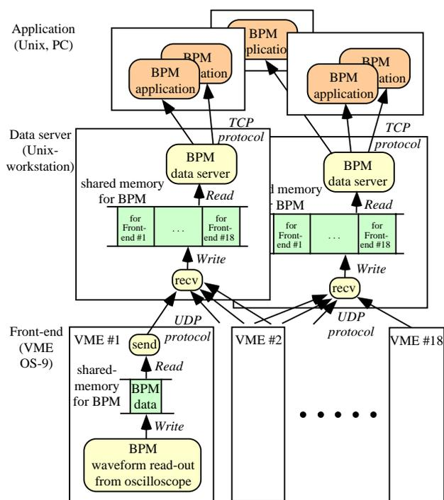
Figure 1: Overview of the data-acquisition system.
