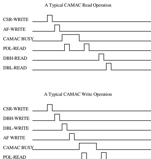
Figure 1. Timing diagram for CAMAC read-and-write operations.
