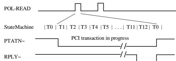
Figure 4. Simplified timing diagram for an 0934 - 0783 transaction
