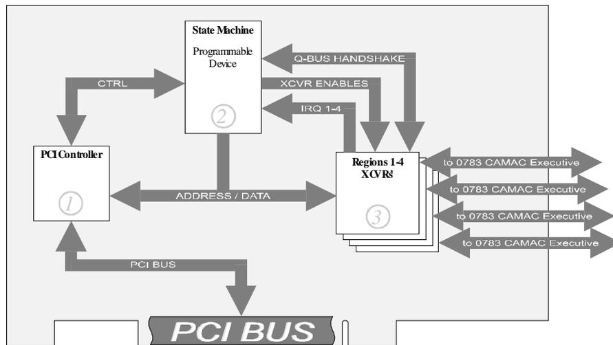
Figure 2. 0934 Module Block Diagram
