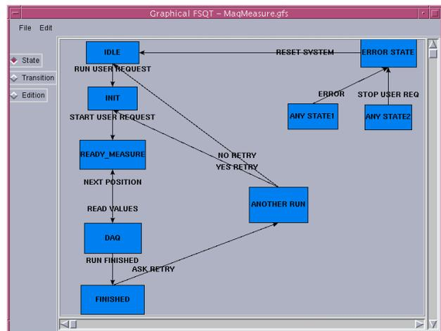
Figure 2. Graphical *FSQT* example.
