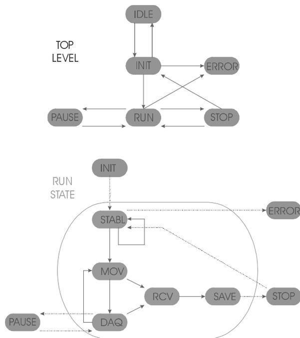
Figure 3. Partial view of the application FSM.
