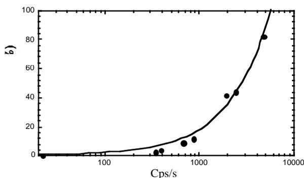
Figure 3: Dead time of the MCA chain as a function of the counting rate
