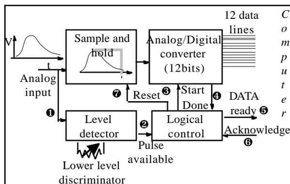
figure 1: Bloc diagram of our MCA interface
