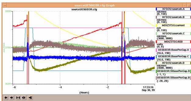
Figure 1: Stability Monitor using StripTool.
