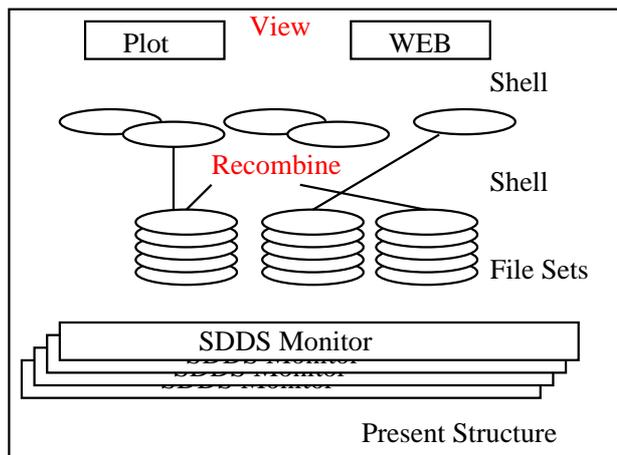
Figure 2: Data Collection and Extraction Engine.
