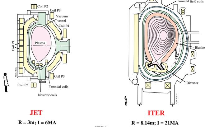
Figure 1 Cross sections of the JET tokamak and of the ITER reactor design
