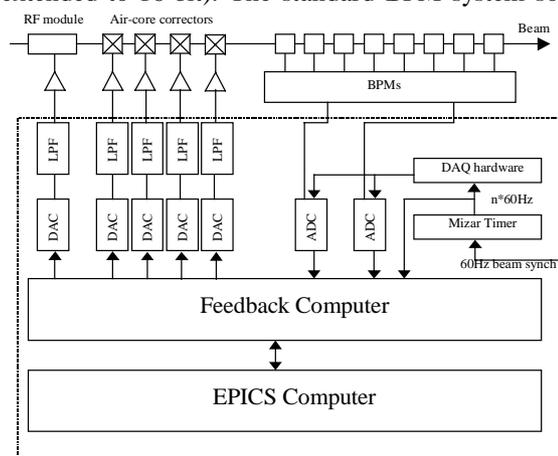
Figure 1. Fast feedback system schematic.
