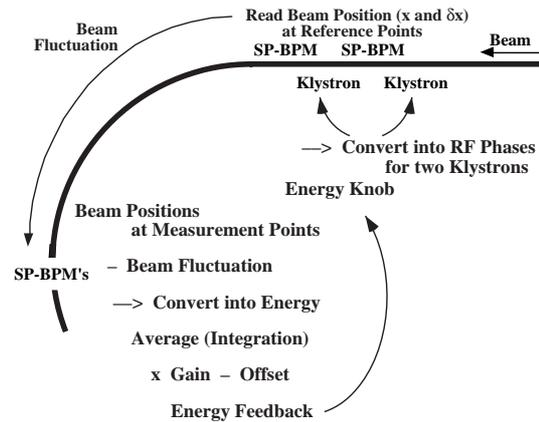
Figure 1: Process flow for beam-energy feedback.
