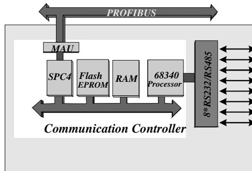
Figure 2: Block diagram of the serial gateway
