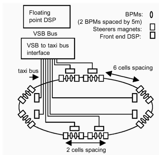
Figure 1: Layout of the global feedback system.
