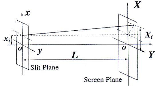
Figure 2: Illustration of  $x'_i$ . L is the distance between the slit plate and the screen.
