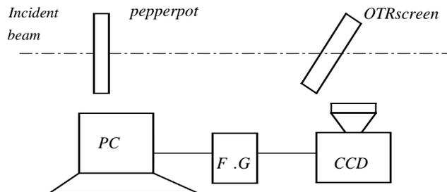
Figure3: Schematic map of the image acquisition system
